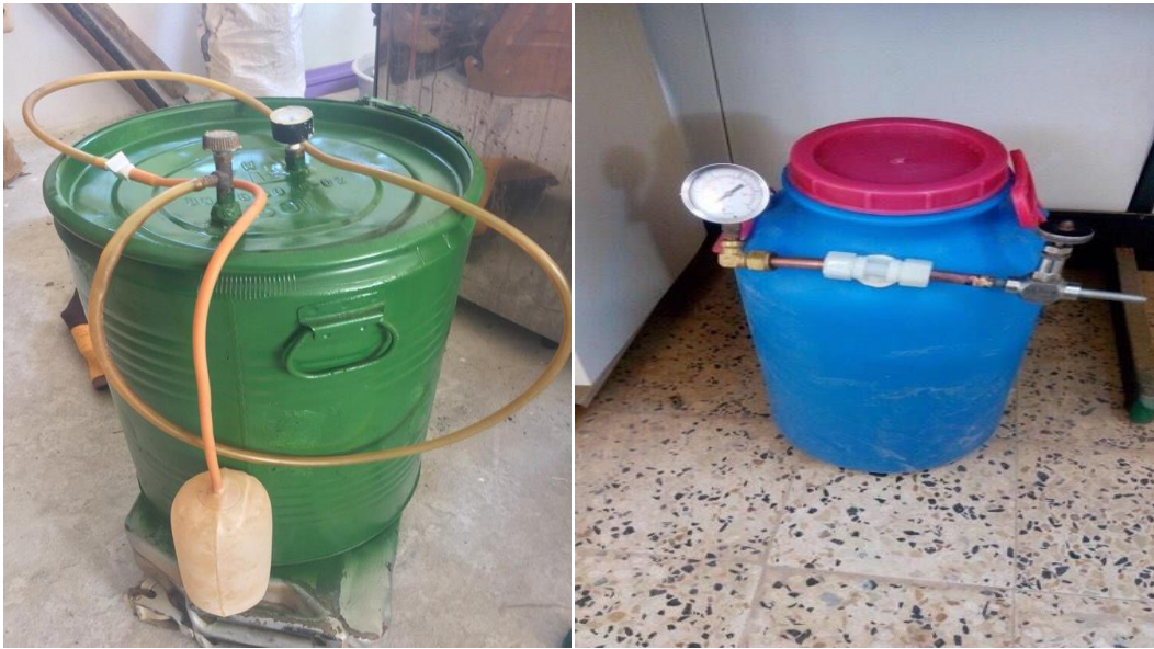
Figure (2): The two plastic and metal digesters
