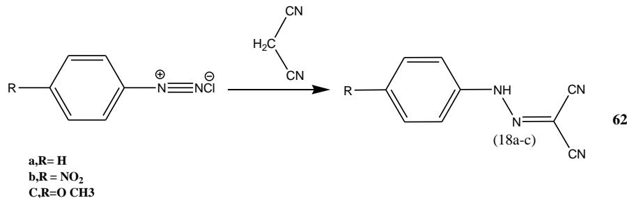
preparation of symmetrical and asymmetrical heterocyclic diazo dyes when aniline derivatives (a-b) were diazotized using sodium nitrite in hydrochloric acid ,the temperature was maintained below 5 °C in an ice bath .The diazotized products were then coupled with malononitrile to give the desired products (a-b ) followed by reflux with hydrazine hydrate in ethanol , the cyclized compound (a-b) was obtained under reflux<sup>[87,88]</sup>
