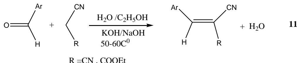
Has been reported as simple effective and rapid Knoevenagel condensation synthesis by using ionic liquid media. The mixture of aromatic aldehyde and dicyanomethane. They were equally carried out in pyridinium salicylate ionic liquid refluxed on 40°C for few minutes occupied the malononitrile derivatives.<sup>[28]</sup>
