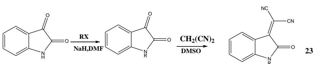
**R**=H, CH<sub>3</sub>, n-Pr,n-hexyl ,PhCH<sub>2</sub>, PhCHCH<sub>3</sub>, 1-(benzotriazole)CH<sub>2</sub>
