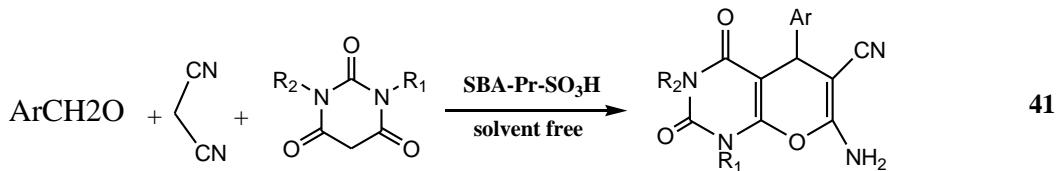
Reaction of the substituted ketones and malononitrile produced enaminonitriles intermediate by the solvent free microwave method with help. The final compounds Synthesized 2-amino-3-cyanopyridines <sup>[58]</sup>
