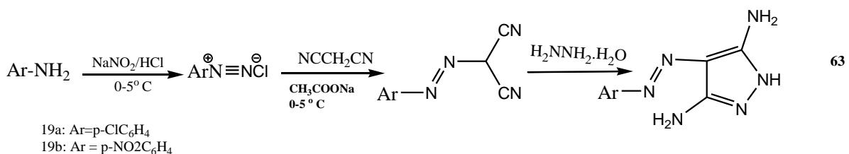
The reaction starts by diazotization of aminobenzoic acid and reaction of the corresponding diazonium salts with malononitrile to give arylazomalononitriles.<sup>[89]</sup>
